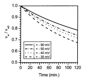
**Figure 10.** Effect of zeta potential on the permeate flux decline. The physico-chemical conditions employed were pressure, 69.0 kPa (10 psi), membrane resistance,  $10^{12}$  m<sup>-1</sup>, particle size, 100 nm, and ionic strength,  $10^{-3}$  M. The cake volume fraction for zeta potential, -30, -40, -50, and -90 mV are 0.449, 0.419, 0.401, and 0.367, respectively.
