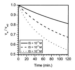
**Figure 9.** Effect of ionic strength on the permeate flux decline. The physico-chemical conditions employed were pressure, 69.0 kPa (10 psi), membrane resistance,  $10^{12} \text{ m}^{-1}$ , particle size, 100 nm, and zeta potential, -30 mV. The cake volume fraction for ionic strength,  $10^{-4}$ ,  $10^{-3}$ , and  $10^{-2} \text{ M}$  are 0.337, 0.449, and 0.538, respectively.
