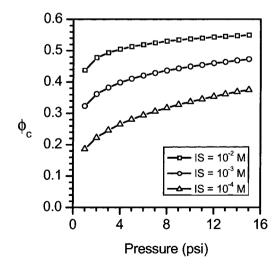
**Figure 7.** Effect of ionic strength on the cake volume fraction. The physico-chemical conditions employed were particle size, 100 nm, and zeta potential, -30 mV.
