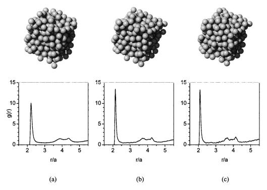
**Figure 3.** The cake structures and the corresponding radial distribution function g(r) for applied pressure (a) 6.9 kPa (1.0 psi), (b) 34.5 kPa (5.0 psi), and (c) 103.4 kPa (15.0 psi). The physico-chemical condition employed are particle radius, 200 nm, zeta potential, -30 mV, and ionic strength,  $10^{-2}$  M. The obtained volume fractions by the simulations are (a) 0.473, (b) 0.530, and (c) 0.571.
