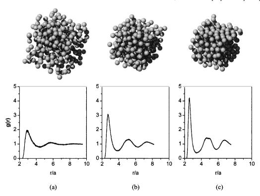
**Figure 2.** The cake structures and the corresponding radial distribution function g(r) for applied pressure (a) 6.9 kPa (1.0 psi), (b) 34.5 kPa (5.0 psi), and (c) 103.4 kPa (15.0 psi). The physico-chemical condition employed are particle radius, 50 nm, zeta potential, -30 mV, and ionic strength,  $10^{-3} \text{ M}$ . The obtained volume fractions by the simulations are (a) 0.147, (b) 0.237, and (c) 0.308.
