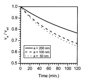
**Figure 8.** Effect of particle size on the permeate flux decline. The physico-chemical conditions employed were pressure, 69.0 kPa (10 psi), membrane resistance,  $10^{12}$  m<sup>-1</sup>, ionic strength,  $10^{-3}$  M, and zeta potential, -30 mV. The cake volume fraction for particle size, 50, 100, and 200 nm are 0.281, 0.449, and 0.554, respectively.
