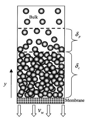
**Figure 1.** Schematic diagram of the concentration polarization and the cake layer in the dead-end membrane filtration. In this diagram  $\delta_p$  and  $\delta_c$  represent the thickness of the concentration polarization and the cake layer, respectively.
