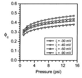
**Figure 5.** Effect of zeta potential on the cake volume fraction. The physico-chemical conditions employed were particle size, 100 nm, and ionic strength,  $10^{-3} \text{ M}$ .
