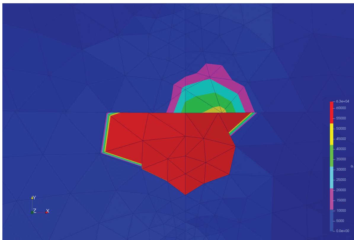
Fig. 12. (Color) Mismatching vertices on an AMI boundary with diverging p values.
