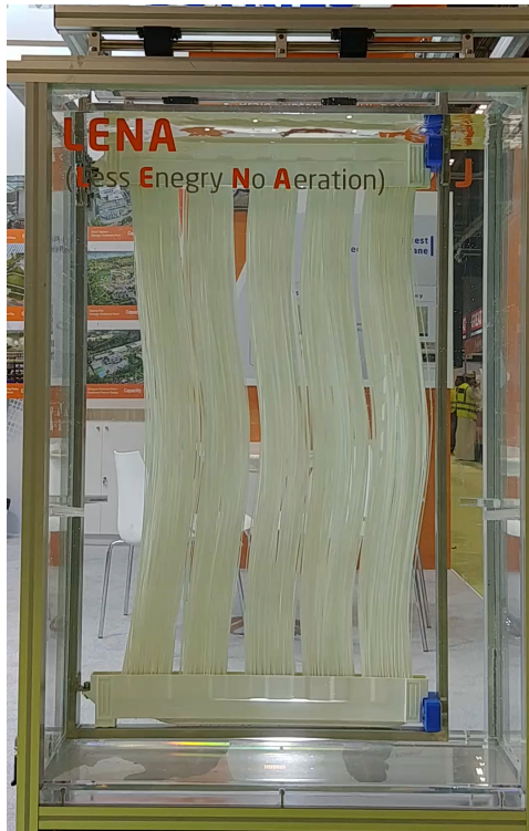
Figure 1: The shaking HF bundle, attached to the ceiling and bottom of the rack surfaces to mitigate particulate fouling on the HF surfaces. ( https://www.coe-pro.com/en/pages/water-plants ).
